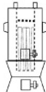
Load dry wood into the stove. Ensure the wood is tightly packed together. The wood should not be above the holes at the top of the fuel chamber.
